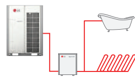
Hot Water+ Underfloor Heating
